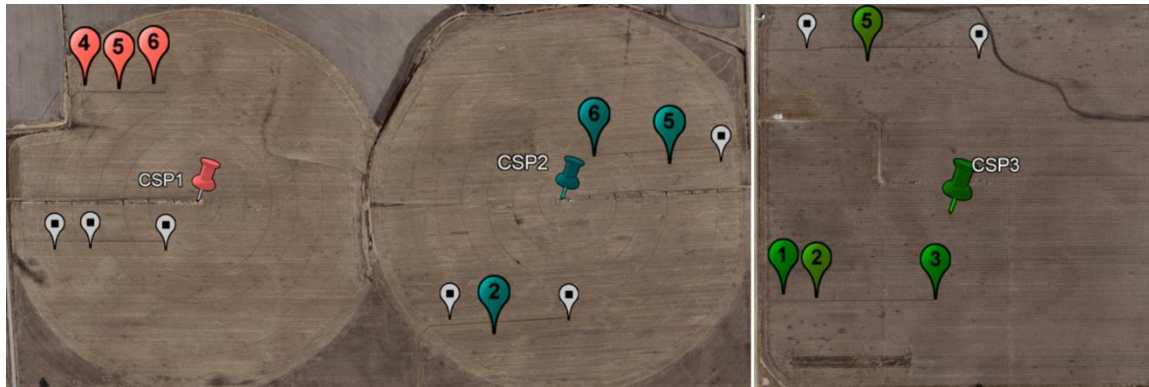
Figure 3. Locations of CRNS and profiles of in-situ soil water content (SWC) time domain reflectometry (TDR) sensors in this study for sites CSP1, CSP2, and CSP3. TDR sensor depths are 10, 25, 50, and 100 cm for all sites and 175 cm for CSP3 only. Field sites CSP1 and CSP2 have three profiles, and CSP3 has four. TDR sensors are denoted with location markers and their associated IMZ number, while the CRNS sensors are denoted with thumbtacks. Gray markers show the IMZs where only vegetation samples are collected and no TDR sensors are present.
