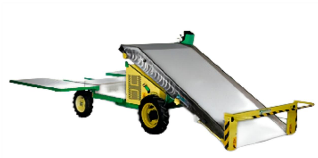
Figure 1(a). SLIDE FW leafy vegetable harvester.
