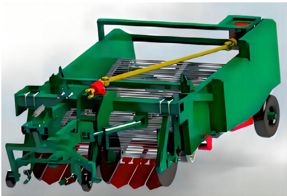
Figure 1(a). SLIDE FW leafy vegetable harvester.
