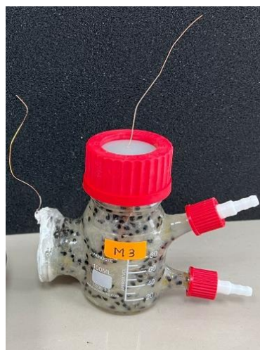
Figure 1. Experimental setup of MFC.
