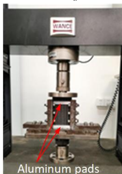
Figure 3. Compression after edge impact test device.
