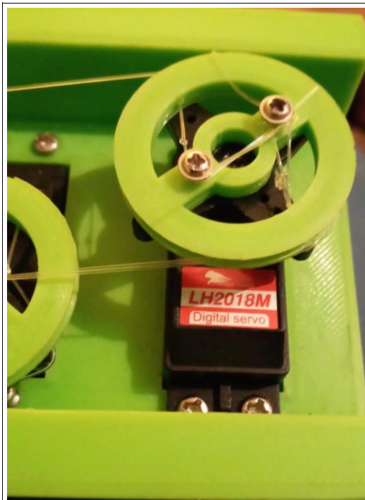
Servomotor and drive pulley for middle, annular, and little fingers
